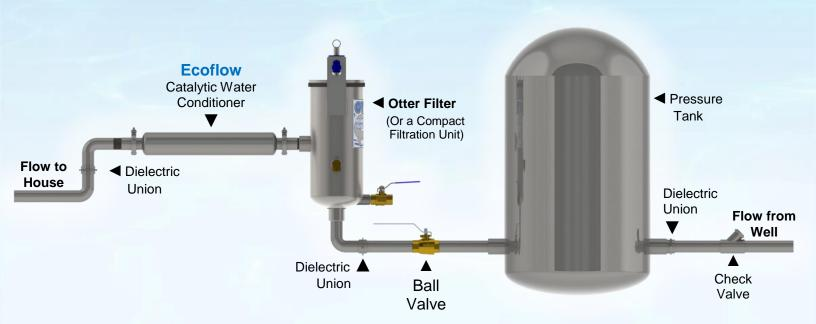
**NOTE:** Dielectric Unions to be installed only if you have Galvanized Supply Lines. Wrap all pipes and fittings for cold weather conditions of 40° F and lower.
